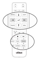
Press the ◀ / ▶ buttons on the keypad to adjust Volume +/-.
