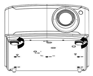
**2.** To lower the level of the projector, lift the projector and twist the adjusters clockwise.
