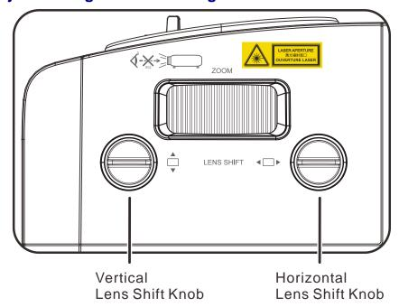
The Lens Shift feature provides a lens shift function that can be used to adjust the position of the projected image either horizontally or vertically within the range detailed below.
