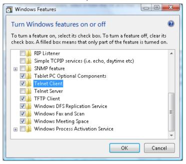
Have "Telnet Client" option checked, then press "OK" button.
