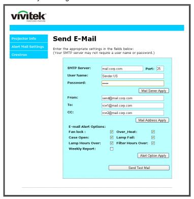
**Note:** Fill in all fields as specified. User can click **Send Test Mail** to test what setting is correct. For successful sending an e-mail alert, you must select alert conditions and enter a correct e-mail address.
